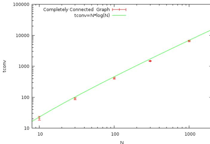
**Fig. 5.** The plot shows the graph coloring in the case of a completely connected graph with  $N$  colors: in this case we find that the convergence turn is  $t_{conv} \sim N \log(N)$ . The points on this graph are averaged on ten algorithm runs.
