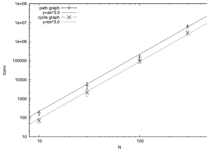
**Fig. 4.** The plot shows the graph coloring in the case of path graphs and special 2-colorable cycle graphs with 2 colors. The convergence turn  $t_{conv}$  of the path graphs and cycle graphs exhibit a power law behavior  $t_{conv} \propto N^{3.0}$ . The cycle graph exhibits a faster convergence. The points on this graph are averaged on ten algorithm runs.
